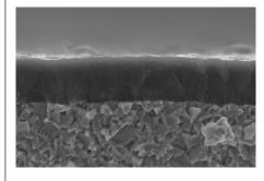
Optimized coating with gradient-sintered tough cemented carbide substrate provides superior wear resistance and exceptional performance for thread turning across a broad range of materials.
